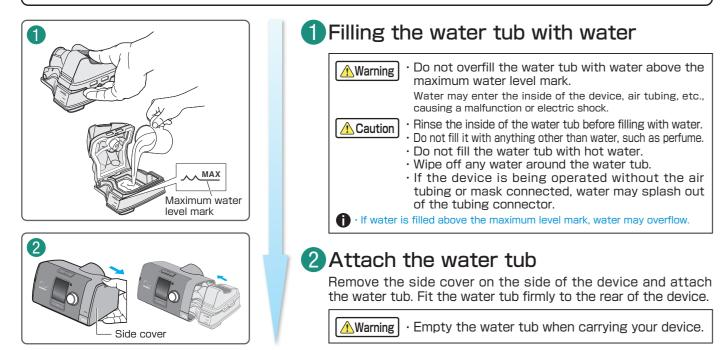
\*Keep the side cover and make sure to operate with the side cover attached to the device when the water tub is not being used.
